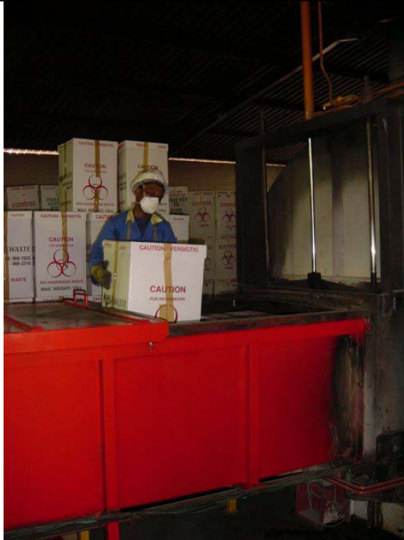
Manual feeding of non-puncture proof cardboard boxes to incinerator
