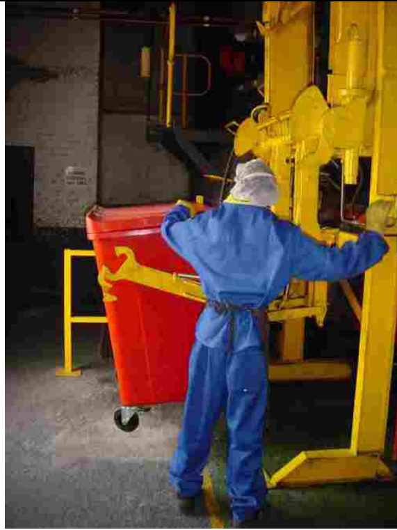
Mechanical lifting of wheelie bins into hopper of incinerator
