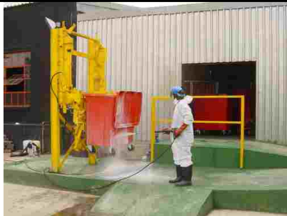
Washing and disinfection of 770 litre wheelie bin
